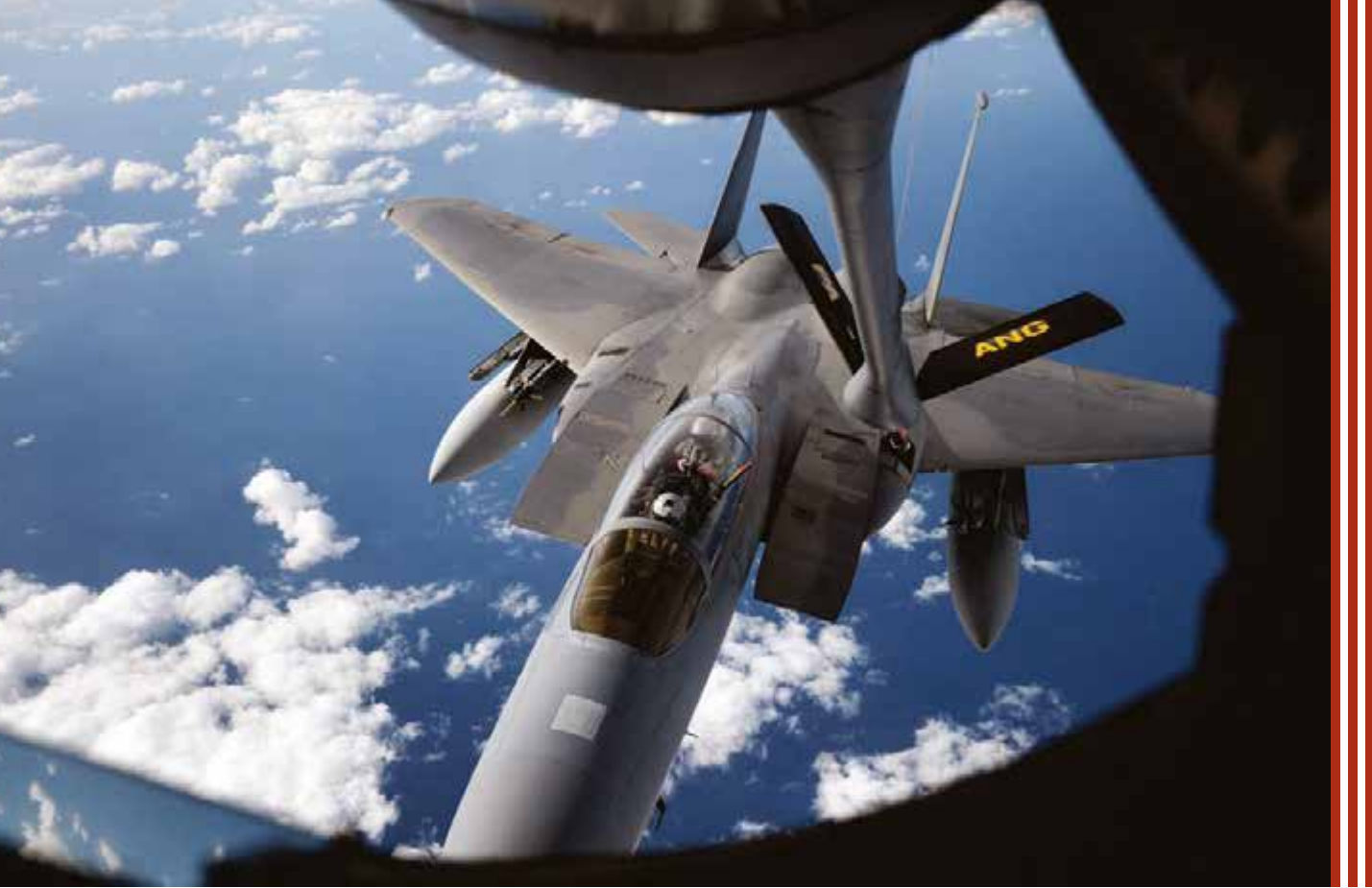
A KC-135 aircraft with the 171st Air Refueling Wing refuels an F-15 aircraft.
