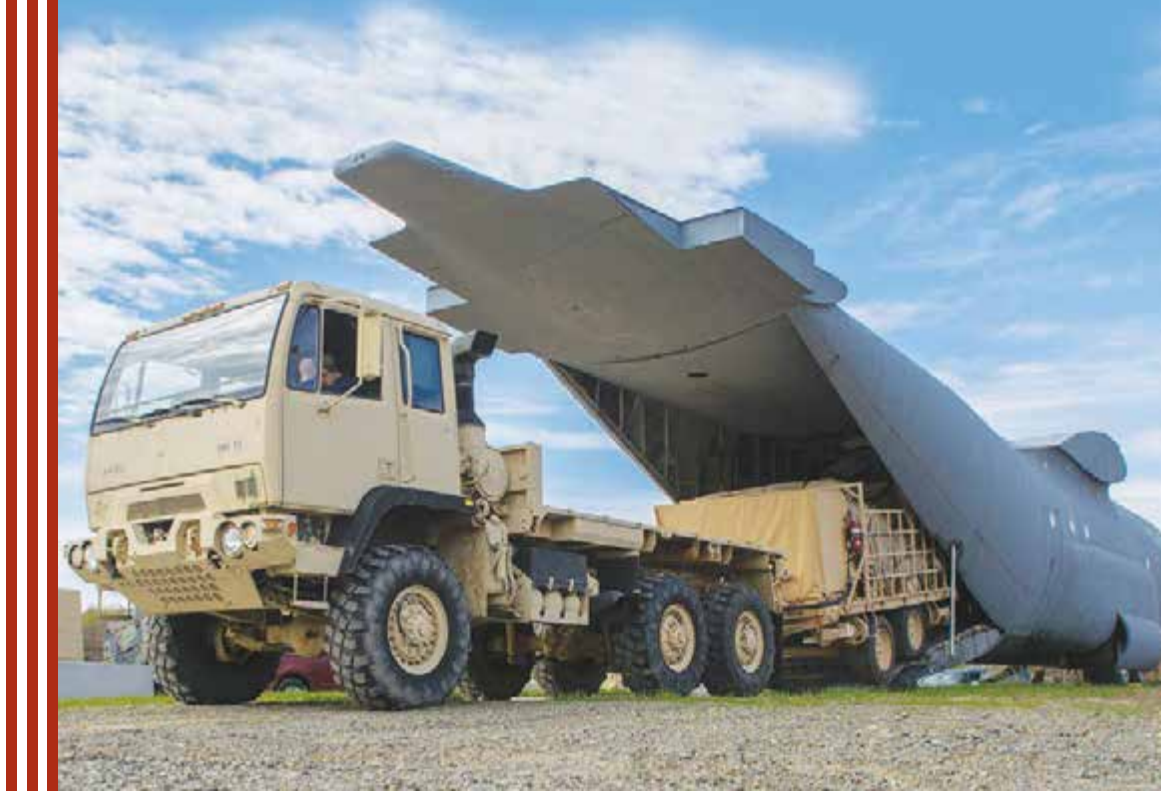
Tobyhanna Army Depot personnel load the Integrated Air and Missile Defense trailer onto a C-130 Hercules aircraft mockup to verify all clearance requirements are met.
